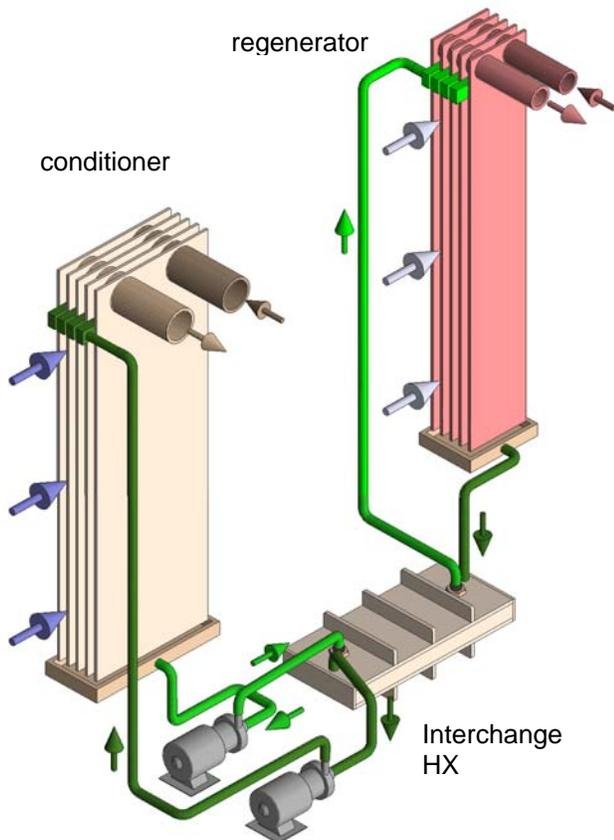
Figure 1 – Operation of a Low-Flow Liquid-Desiccant Air Conditioner
